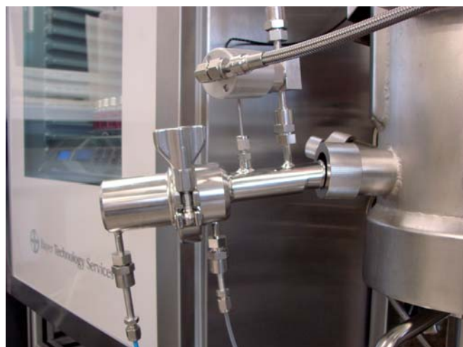
BaychromAT® SamplingValve integrated into the INGOLD port of a steel fermenter
