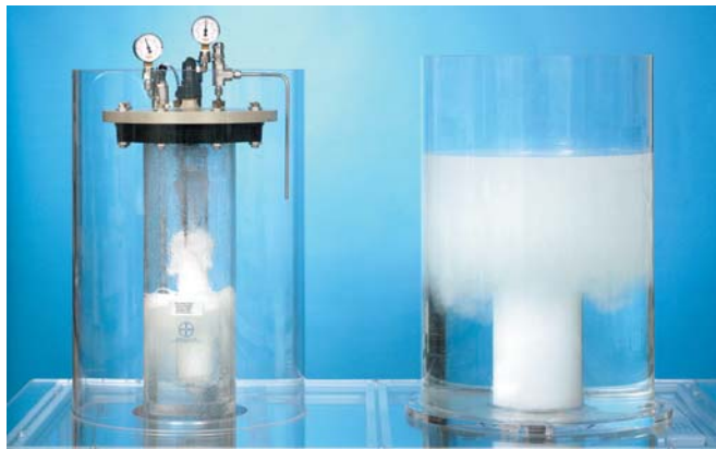
Lab unit for air saturation and bubble size distribution testing
