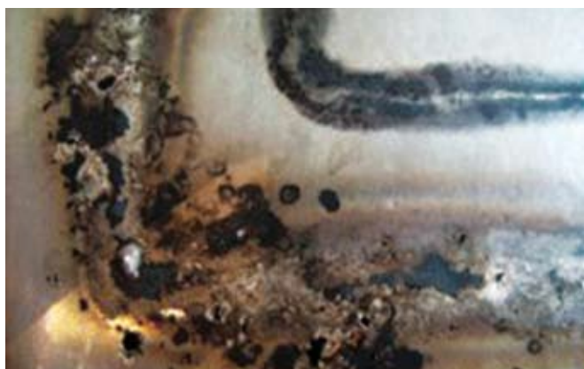
Crevice Corrosion in the Vicinity of Welding Seams
