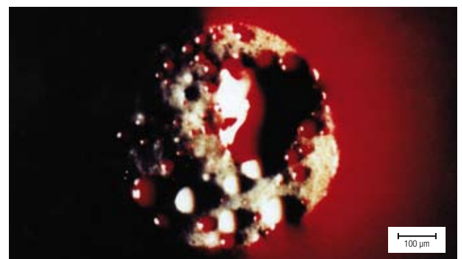
Crater in a coated surface (light microscopy image)
